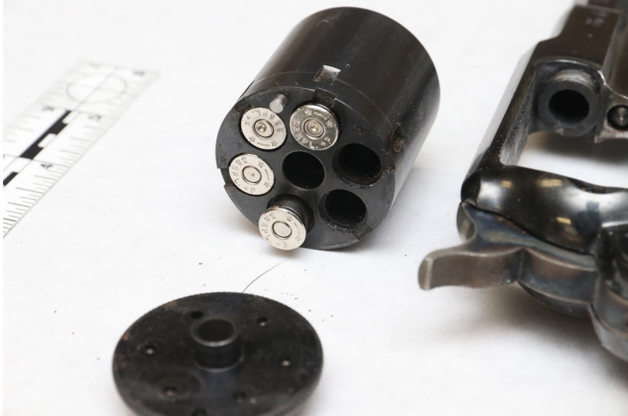
Watson's pistol cylinder. Two cartridges are fired and two remain unfired.
