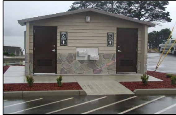
Photo 10-7 Precast concrete flush restroom
