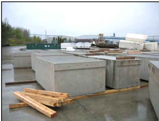
Photo 5-7 Individual concrete float sections
