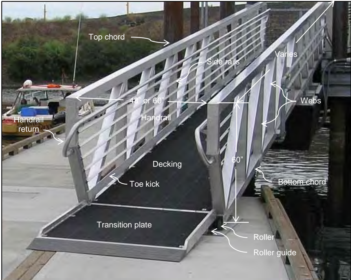
Photo 7-8 Gangway design components
