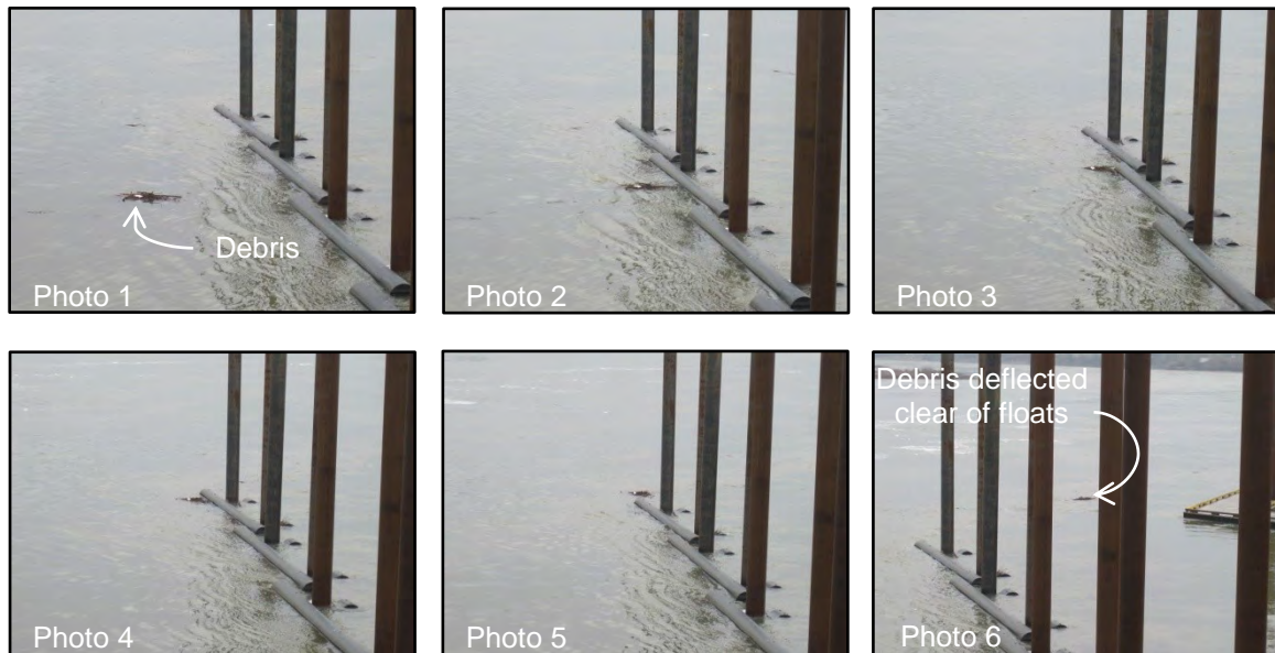
Photo 8-6 Progression of debris as it approaches, engages, and leaves the debris deflection boom
