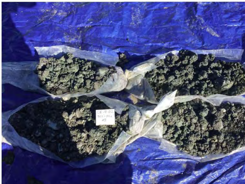
Photo 6 – View of material recovered during drilling boring CE-18-01 from 30' to 40'.
