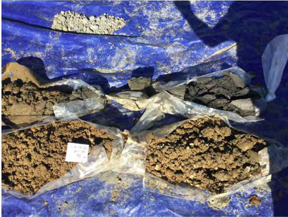
Photo 9 – View of material recovered during drilling boring CE-18-01 from 60' to 70'.
