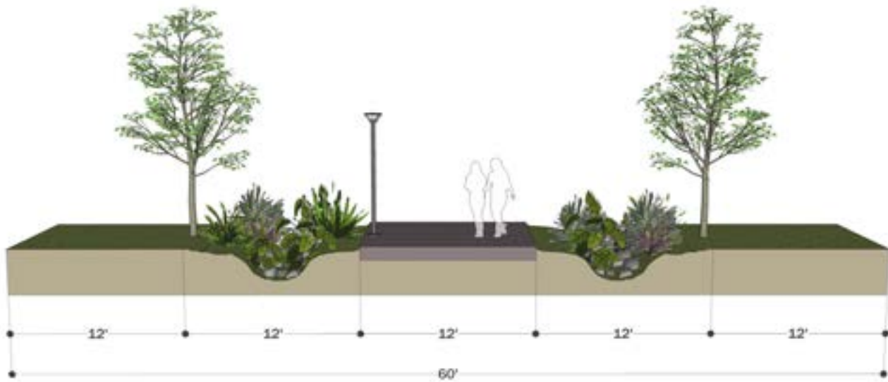
Cross Section of the Pedestrian-Bike Spine (at maximum width)
