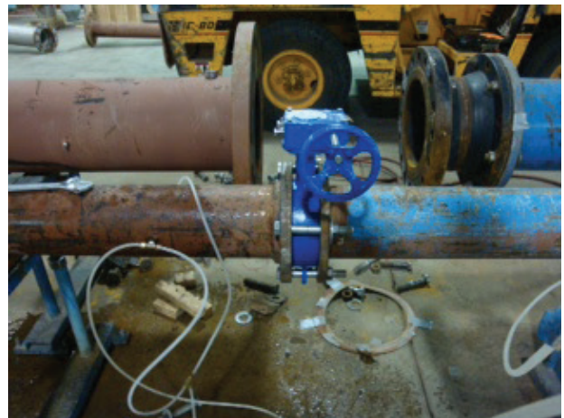
BF Series Wafer / Lug Butterfly Valves being tested at an independent research laboratory
