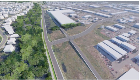
The 122nd Tie-in is designed to preserve the long-term diamond interchange footprint and allow phased construction of the ultimate mainline expressway and bridge over the crossroad.
