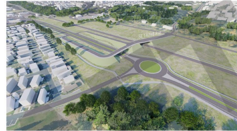
This tie-in allows the consolidation of left-turn access to/from OR 212/224 through the development of a grade-separated overcrossing of the highway and new Sunrise Gateway Corridor and provides a gateway to the industrial site.
