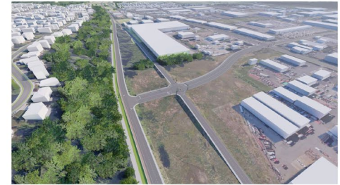
The 122nd Tie-in is designed to preserve the long-term diamond interchange footprint and allow phased construction of the ultimate mainline expressway and bridge over the crossroad.
