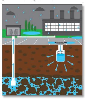
A UIC releases stormwater underground; water wells pull groundwater for drinking and other uses.
