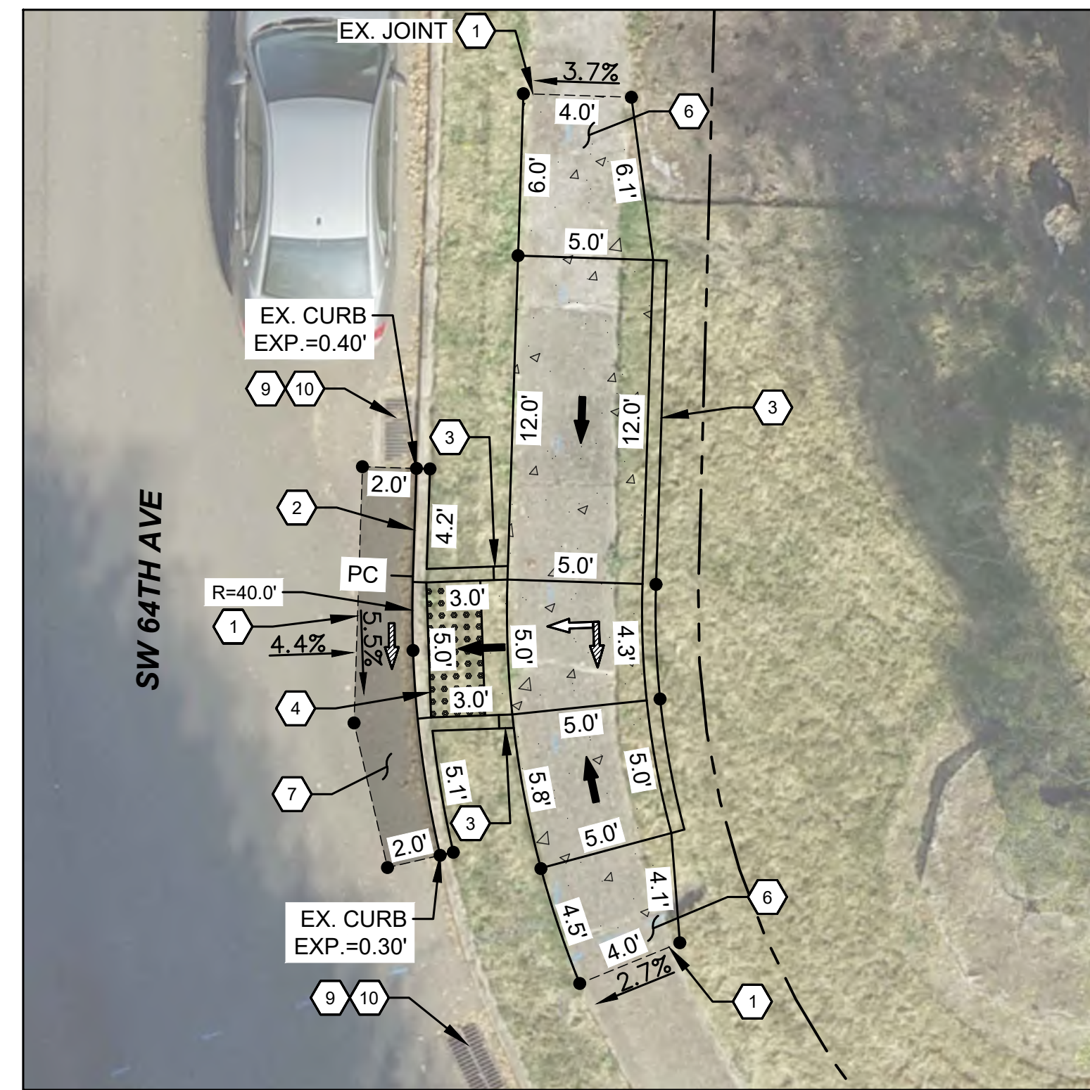
NE CORNER - COMBINATION RAMP 1" = 5'
