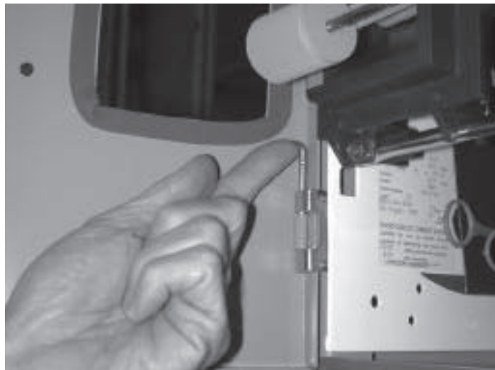
Figure 28. Hinge Pin Removal
