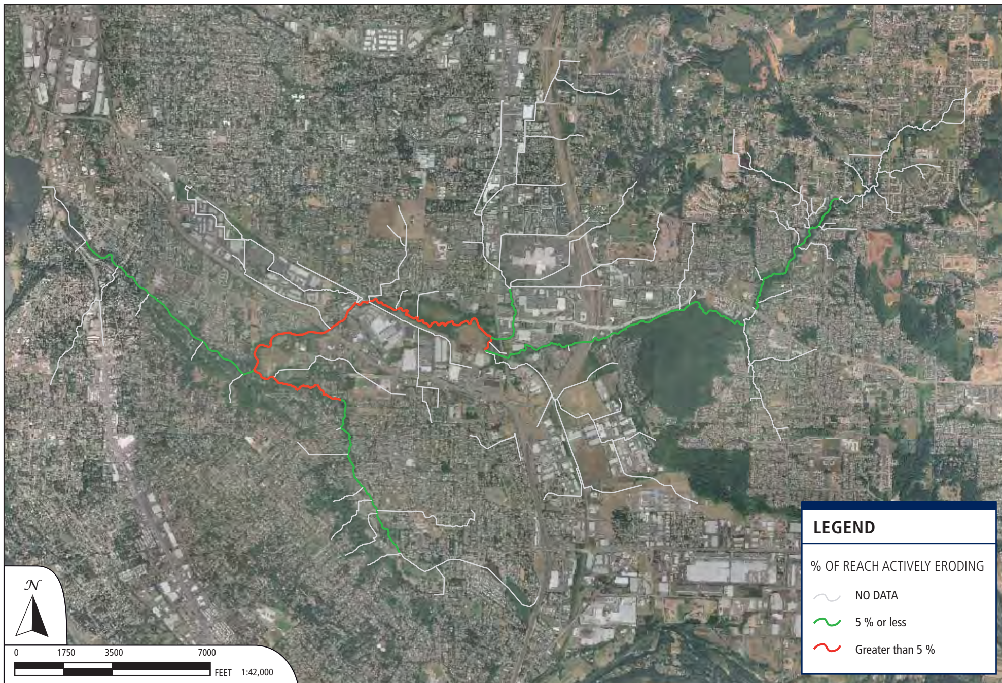
Figure 2-15 Kellogg/Mt. Scott - At Risk Channels due to Bank Erosion WES WATERSHED ACTION PLAN
