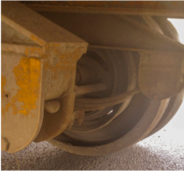
Rubber worn down to the wheel.
