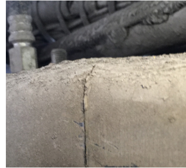
Cracked truck frame.
