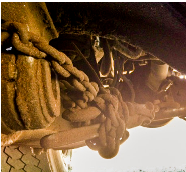
Chain and binder in a crisscross pattern holding together walking beam suspension system.
