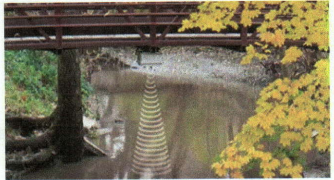
The first stream sensor developed by IFC researchers and students was installed on Ralston Creek in Iowa City.
