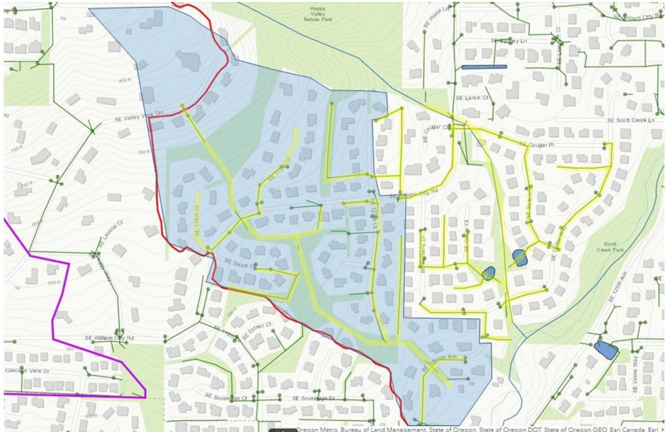
Figure 1: Estimate of Study Area draining through SE 121st Court and downstream to Mt. Scott Creek, along with adjacent storm sewer system to be included in the hydraulic model
