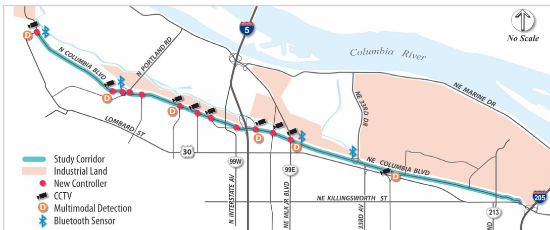
Location of ITS devices along Columbia Blvd
