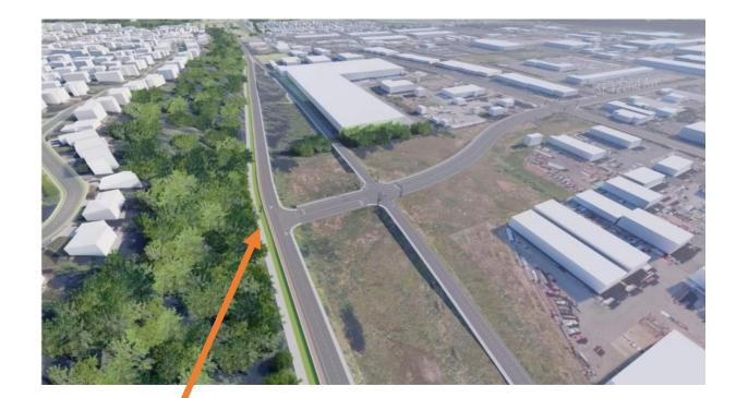
122nd tie-in provides one-way couplet with two-phase signal operation at the long-term ramp locations, while a multi-use path connects to Highway 212 on the east side of SE 122nd Avenue.
