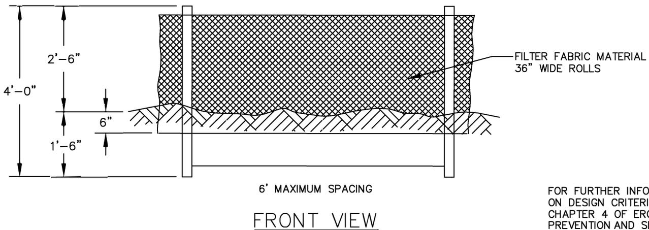
FOR FURTHER INFORMATION ON DESIGN CRITERIA SEE CHAPTER 4 OF EROSION PREVENTION AND SEDIMENT CONTROL PLANNING AND DESIGN MANUAL.
