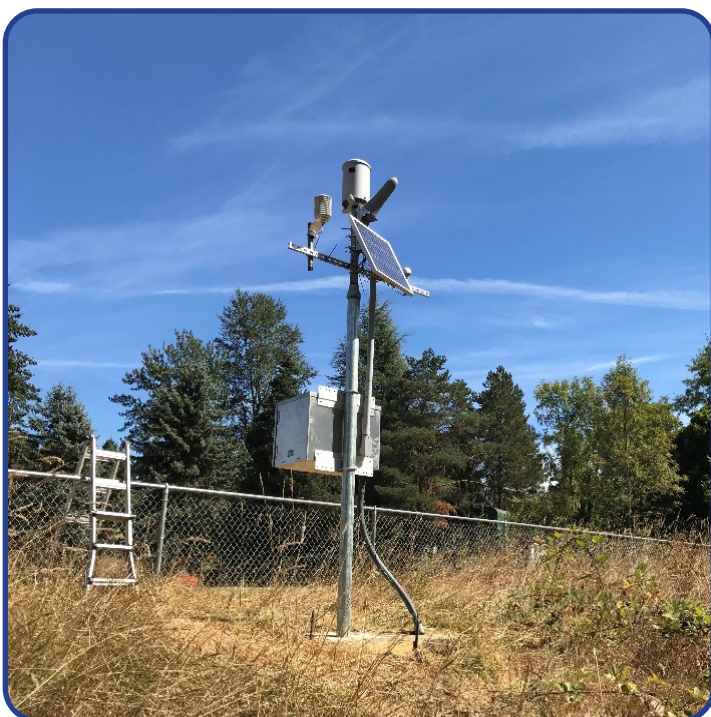
Image 4: Kellogg Creek at Rowe Middle School gage after precipitation upgrade
