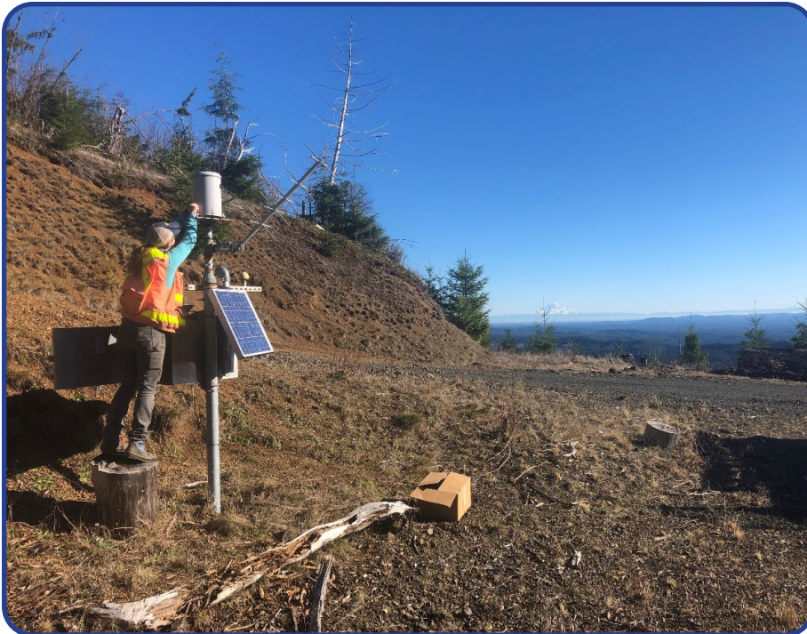
Image 5: WEST technician performing maintenance on a Chehalis River Basin Flood Warning precipitation gage.
