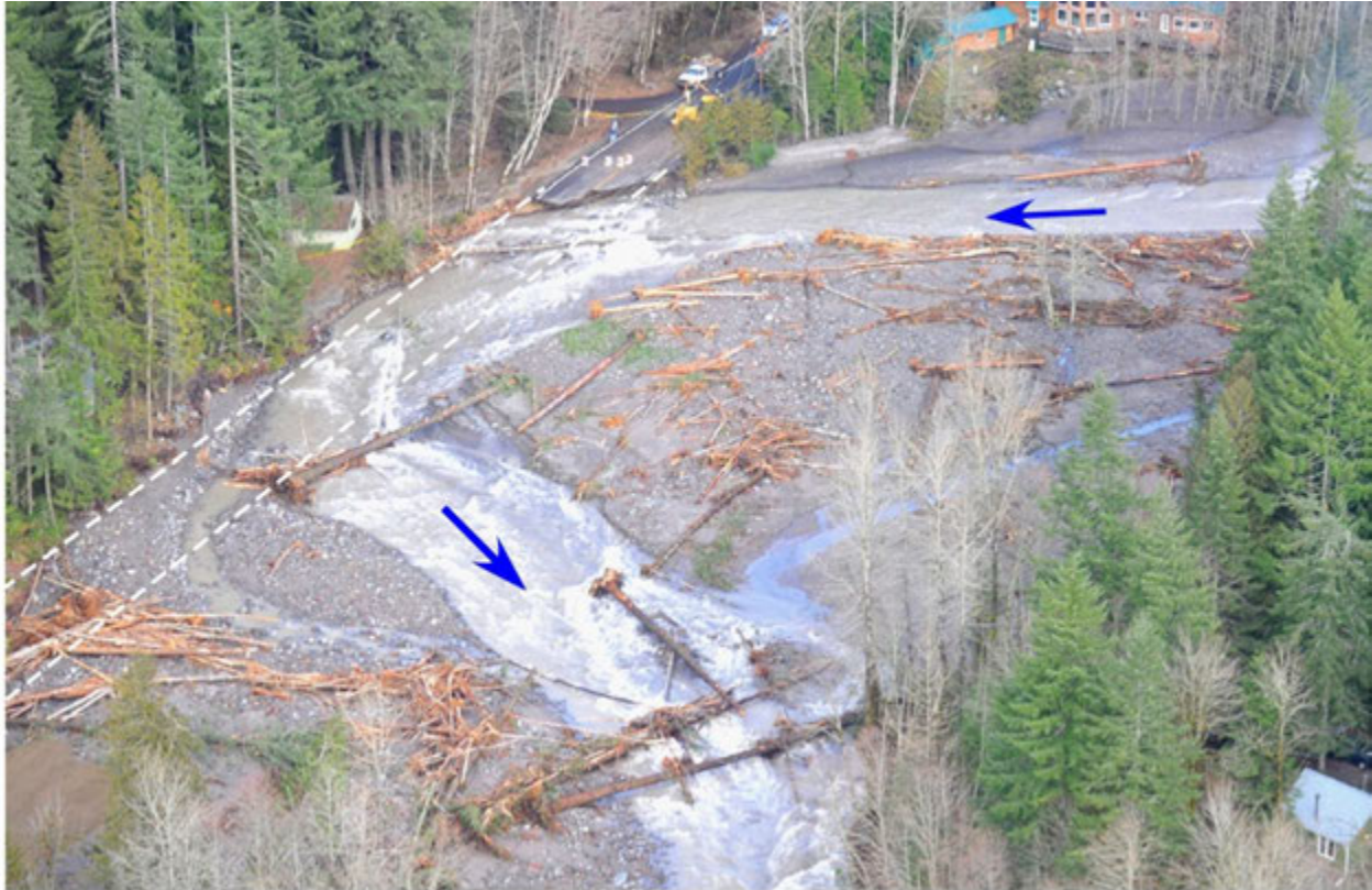
Figure 32. Upper Sandy RM 44.1 Lolo Pass Road washout in 2011. The channel moved through the road adding over 60 ft to its migration zone. The flood left a net increase in the quantity of wood in the channel which added additional flow resistance and enhanced fish habitat. Historic confinement and wood clearing has concentrated the river's energy and severely limited the formation of beneficial salmon habitat. Providing the river with more room to move and implementing flood protection measures that focus on energy dissipation will not only improve habitat but reduce long-term flood protection costs. In this case the road was rebuilt in its pre-existing location.
