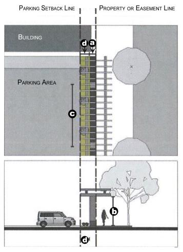
Examples of Low Wall & Trellis Screening: The trellis portion of the screen provides opportunities for increased shade and extends the feeling of a built edge along the sidewalk. The low wall provides a sense of physical separation from cars and can serve as informal seating.
