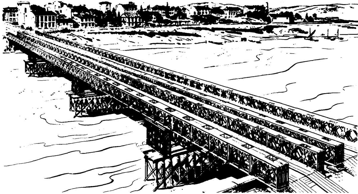
Figure 17-1 Two continuous-panel bridges with panel crib piers on pile piers
