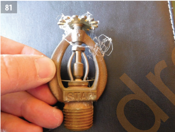
Star-manufactured sprinkler head found in the spare-sprinkler-head cabinet.
