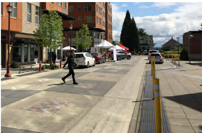
Curbless streets with shared traffic and opportunities for festival closures, street seat parklets, and other amenities. (Beacon Hill neighborhood - Seattle, WA)
