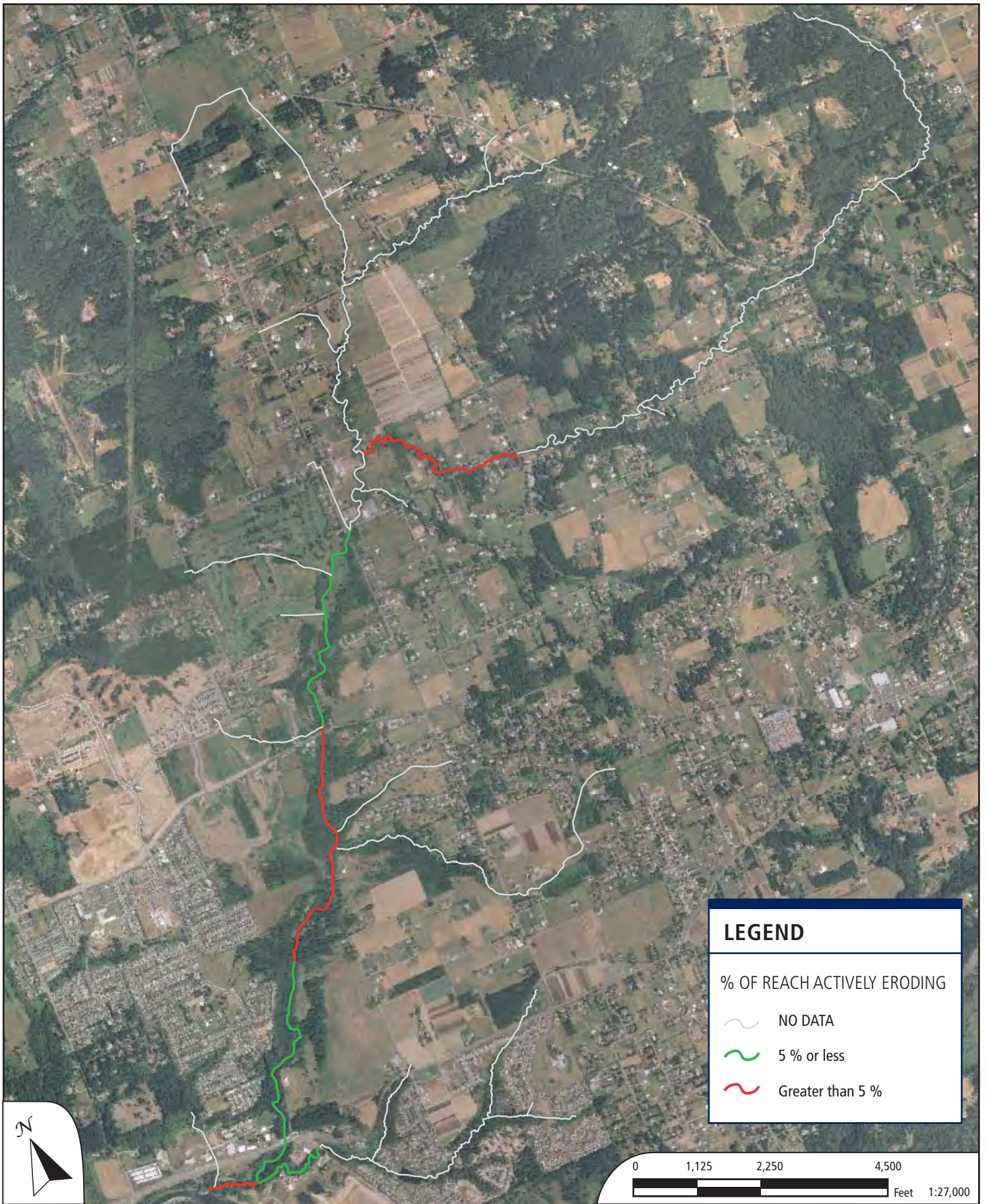
Figure 2-14 Rock Creek - At Risk Channels due to Bank Erosion WES WATERSHED ACTION PLAN
