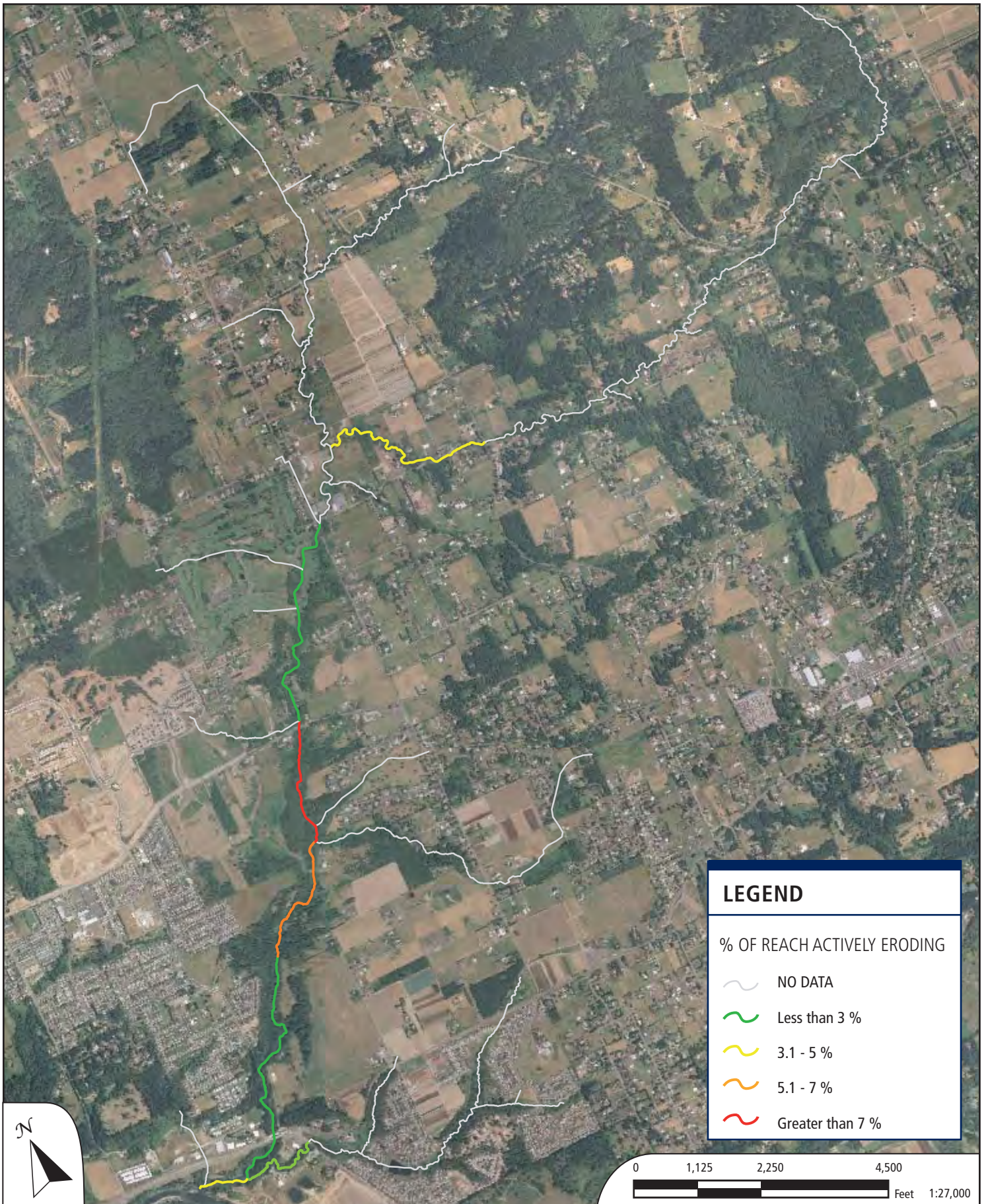
Figure 2-11 Rock Creek - Bank Erosion by Reach WES WATERSHED ACTION PLAN
