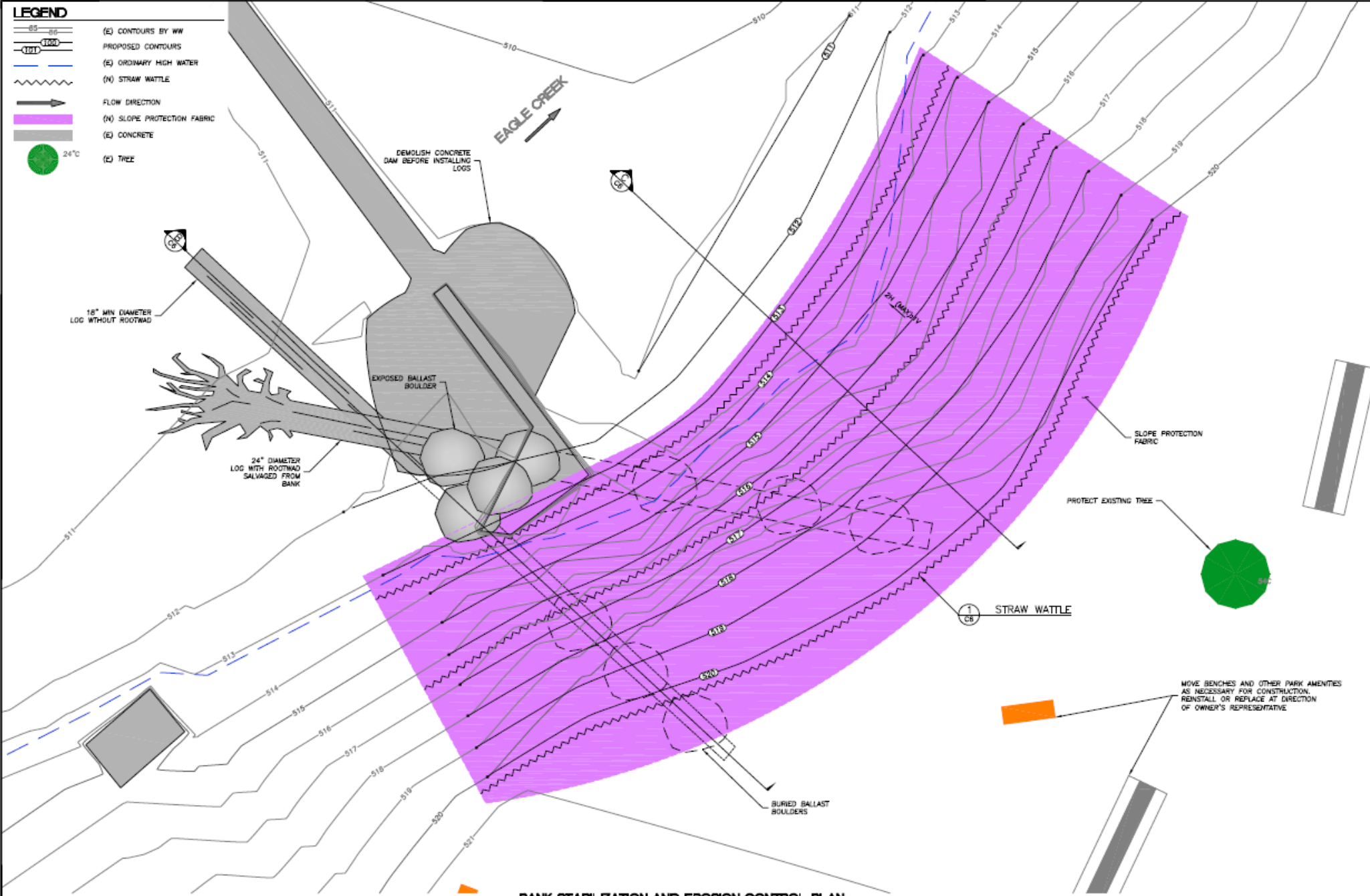
BANK STABILIZATION AND EROSION CONTROL PLAN SCALE: 1" = 3'
