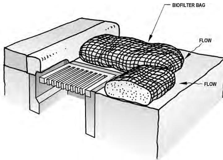
Inlet Protection – Biofilter Bags Around Catch Basin
