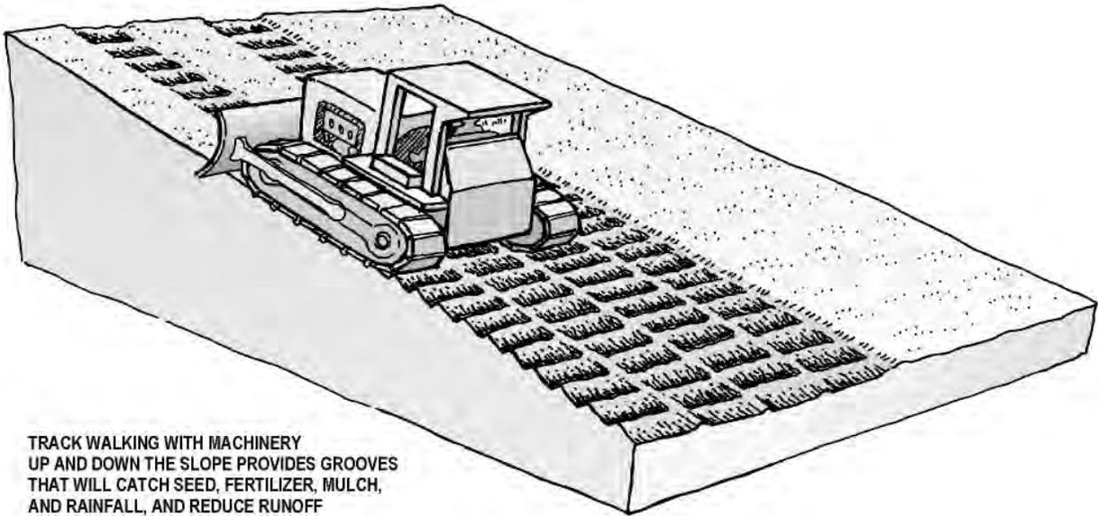
Leaving the slopes in a roughened condition after clearing or creating a rough soil surface with horizontal depressions or grooves will trap seed and reduce runoff velocity. Roughening can be accomplished by ‘track walking’ slopes with tracked equipment, by using a serrated wing blade attached to the side of a bulldozer, or by other agricultural equipment.
