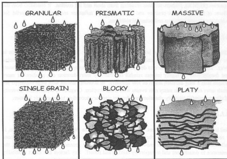
Figure 2-3 Soil Structure
