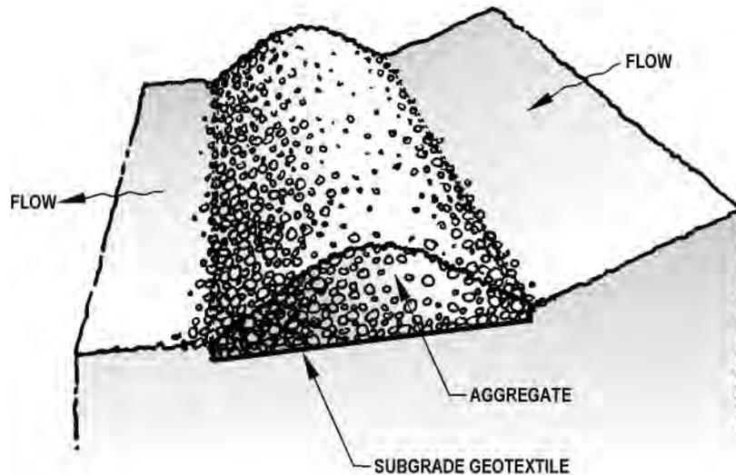
**AGGREGATE BERM** - Retains sediment in gravel or crushed rock berm.
