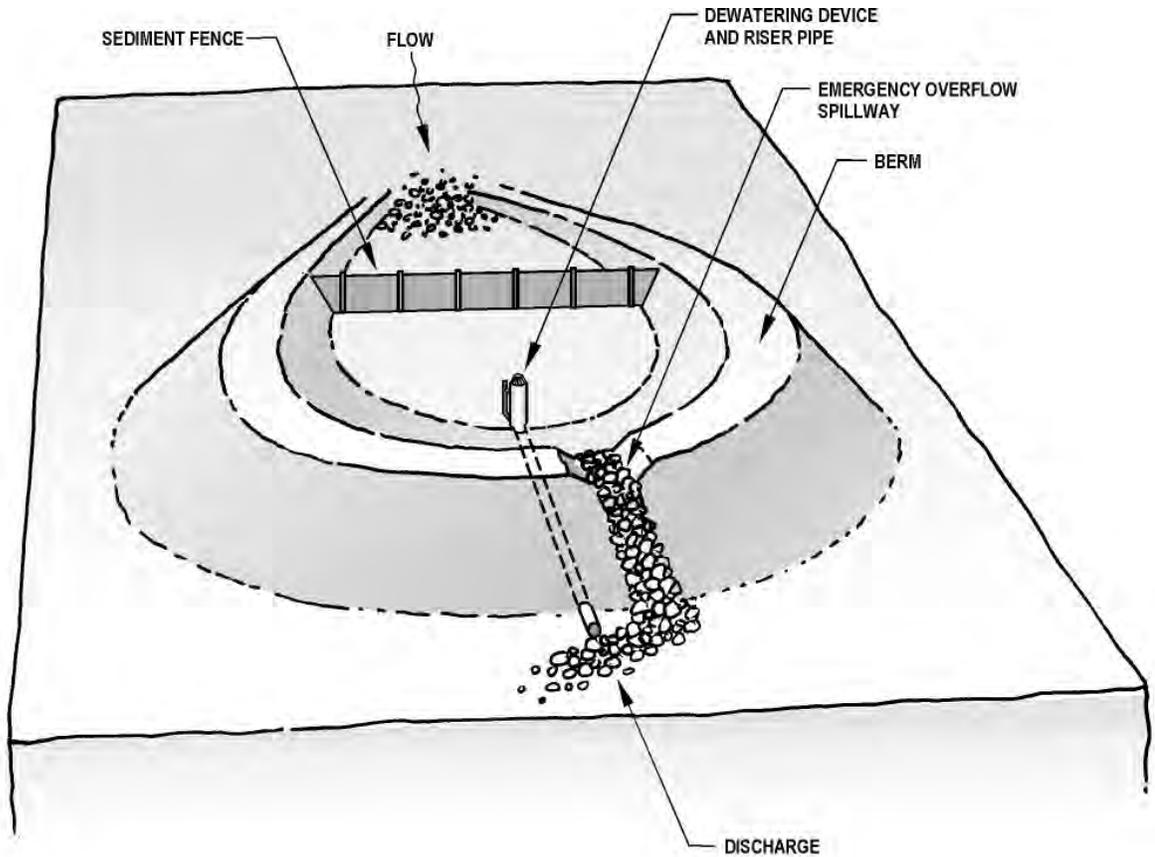
A temporary sediment basin has one or more inflow points and baffles to spread the flow, wet storage and dry storage, a securely anchored riser pipe, a dewatering device and an emergency overflow spillway. The sediment basin serves drainage areas less than 10 acres and has a design life of approximately 1-year.
