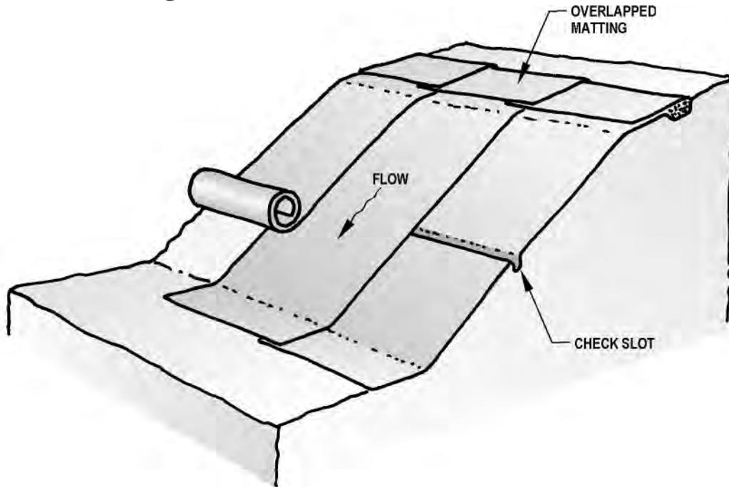
There are numerous erosion control products available that can be described in various ways, such as matting, blankets, fabric and nets. We will call them all matting. A wide range of materials and combination of materials are used to produce matting including, but not limited to: straw, jute, wood fiber, coir (coconut fiber), plastic netting, and Bonded Fiber Matrix. The selection of matting materials for a site can make a significant difference in the effectiveness of the BMP.
