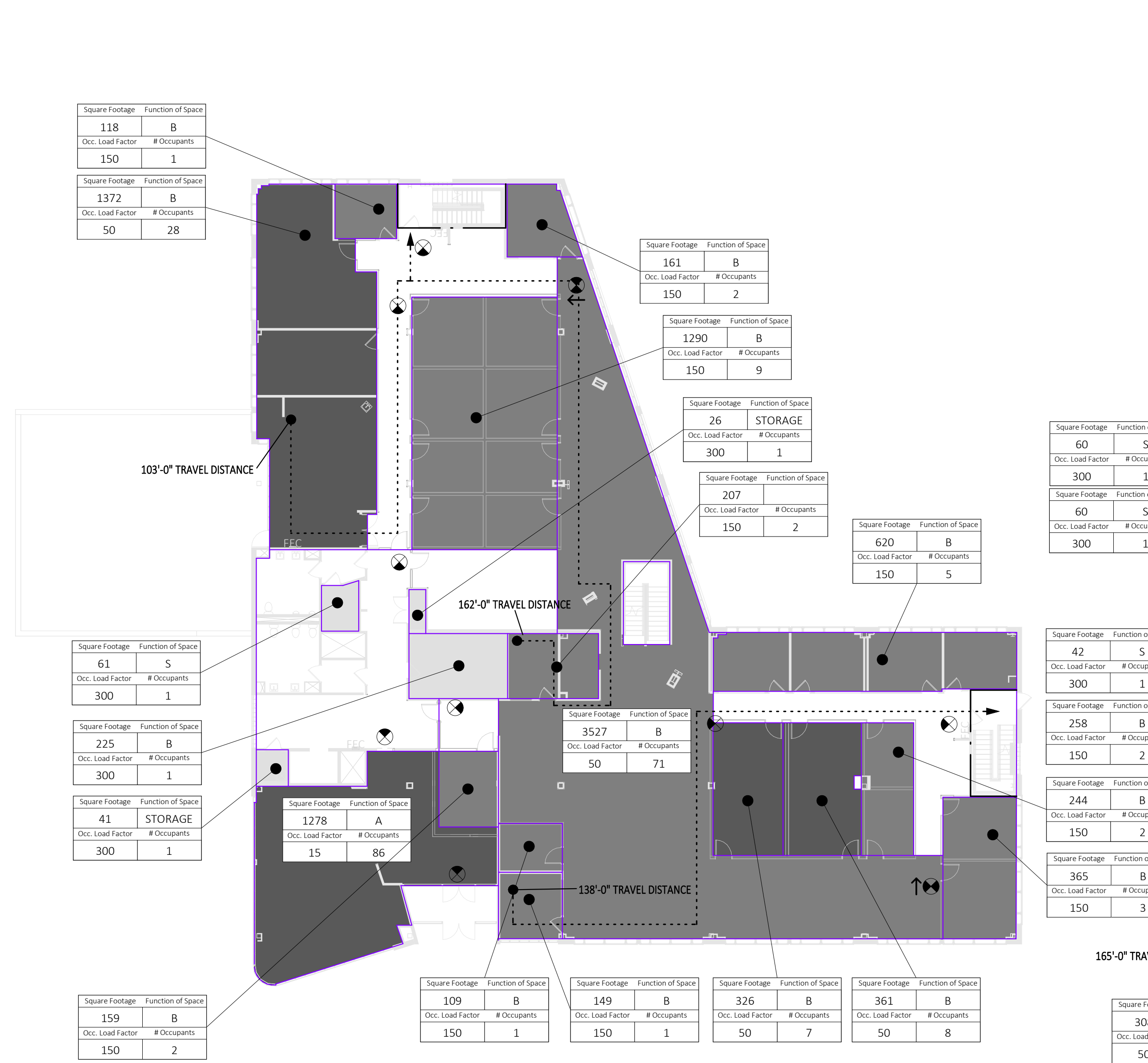
2 LEVEL 01 - OCCUPANT LOAD 1/16" = 1'-0"
