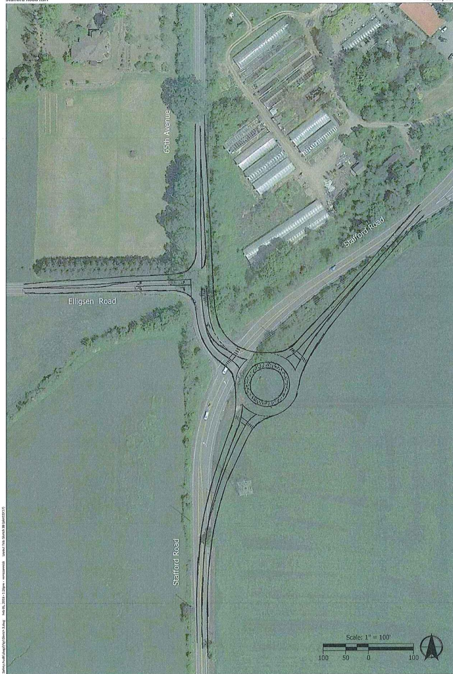
Stafford Road/65th Avenue - Roundabout Concept and 65th Avenue/Elligsen Road - Turn Lane Concept Clackamas County, Oregon
