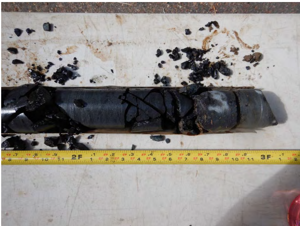
B: Boring LT-2, Sample R-4, Depth 40.5-43.5 ft. Image 3 of 3.
