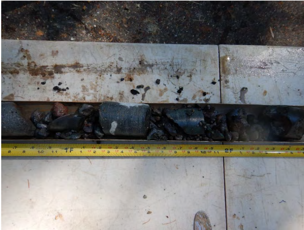
A: Boring LT-2, Sample R-1, Depth 30.0-33.0 ft. Image 2 of 3.
