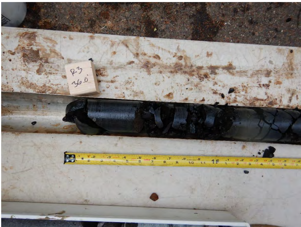
B: Boring LT-2, Sample R-3, Depth 36.0-40.5 ft. Image 1 of 4.
