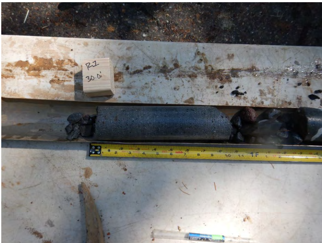
B: Boring LT-2, Sample R-1, Depth 30.0-33.0 ft. Image 1 of 3.
