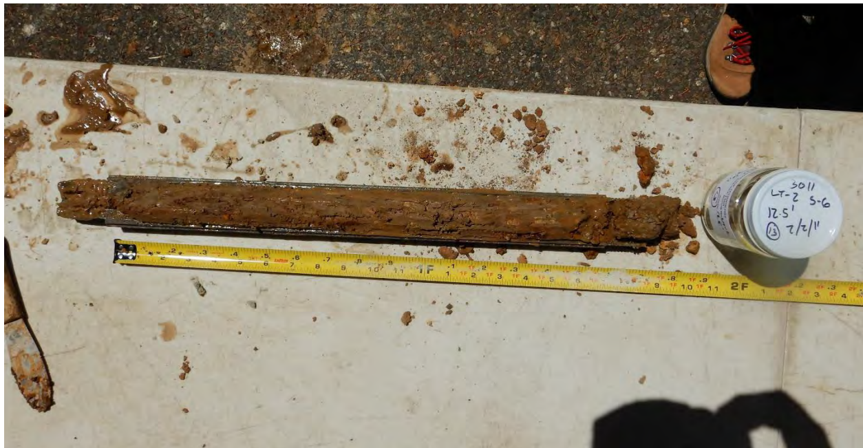
B: Boring LT-2, Sample S-6, Depth 15.0-16.5 ft. Note: Depth is mislabeled on sample jar in image.
