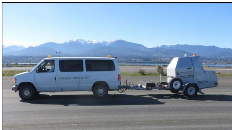
Figure 2 – KUAB 150 Falling Weight Deflectometer
