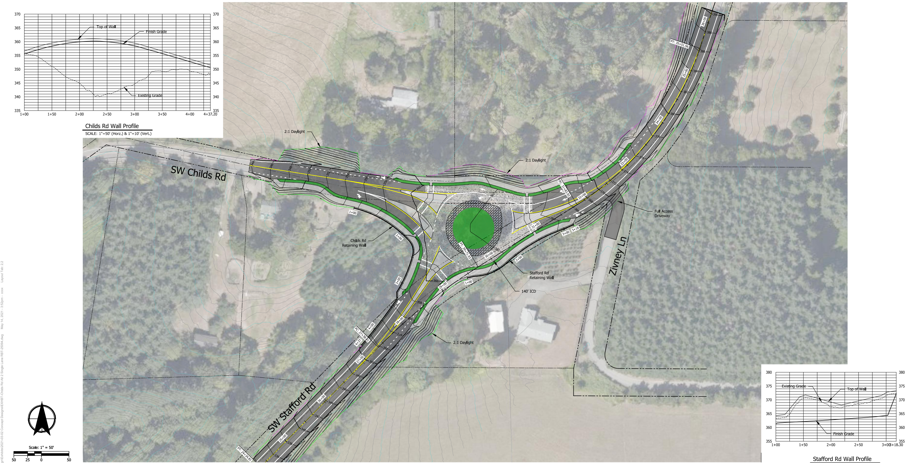
Figure 10: SW Childs Rd Alternative 2.2 - Roundabout
