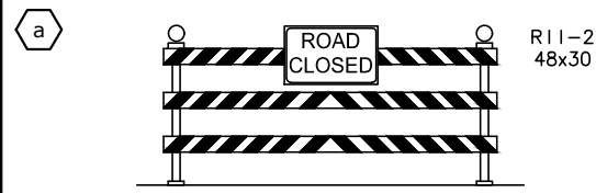
TEMPORARY TYPE 3 BARRICADE SCALE: NTS
