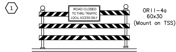
TEMPORARY TYPE 3 BARRICADE SCALE: NTS
