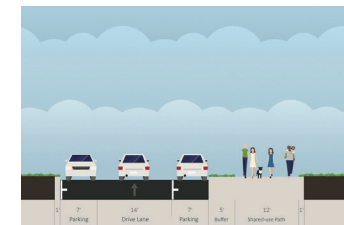
A Proposed cross section for Monroe Street, Linwood to 72nd Avenue (bike/ped path)
