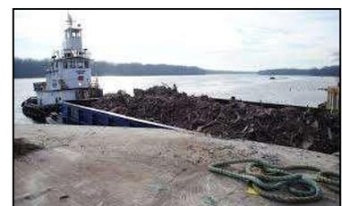
environmentally sensitive area. The trucks will stage debris to be loaded onto the barge, and then the barge will bring the debris across the river. A grapple device will be utilized to unload the debris and reload the debris back onto another truck to be transported to the appropriate TDSRS or final disposal location.
