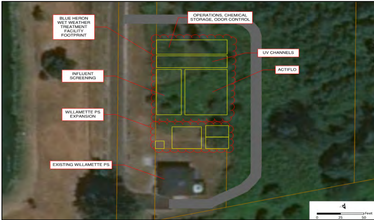
Figure 6.18 Scenario 4: Blue Heron Wet Weather Facility Potential Layout
