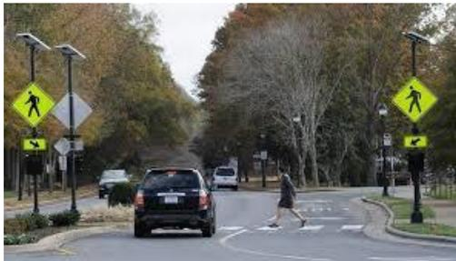
**Figure 14: Example of an advance warning beacon**
