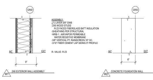
ASSEMBLY: FOUNDATION WALL 6" CONCRETE FOUNDATION WALL PER STRUCTURAL
