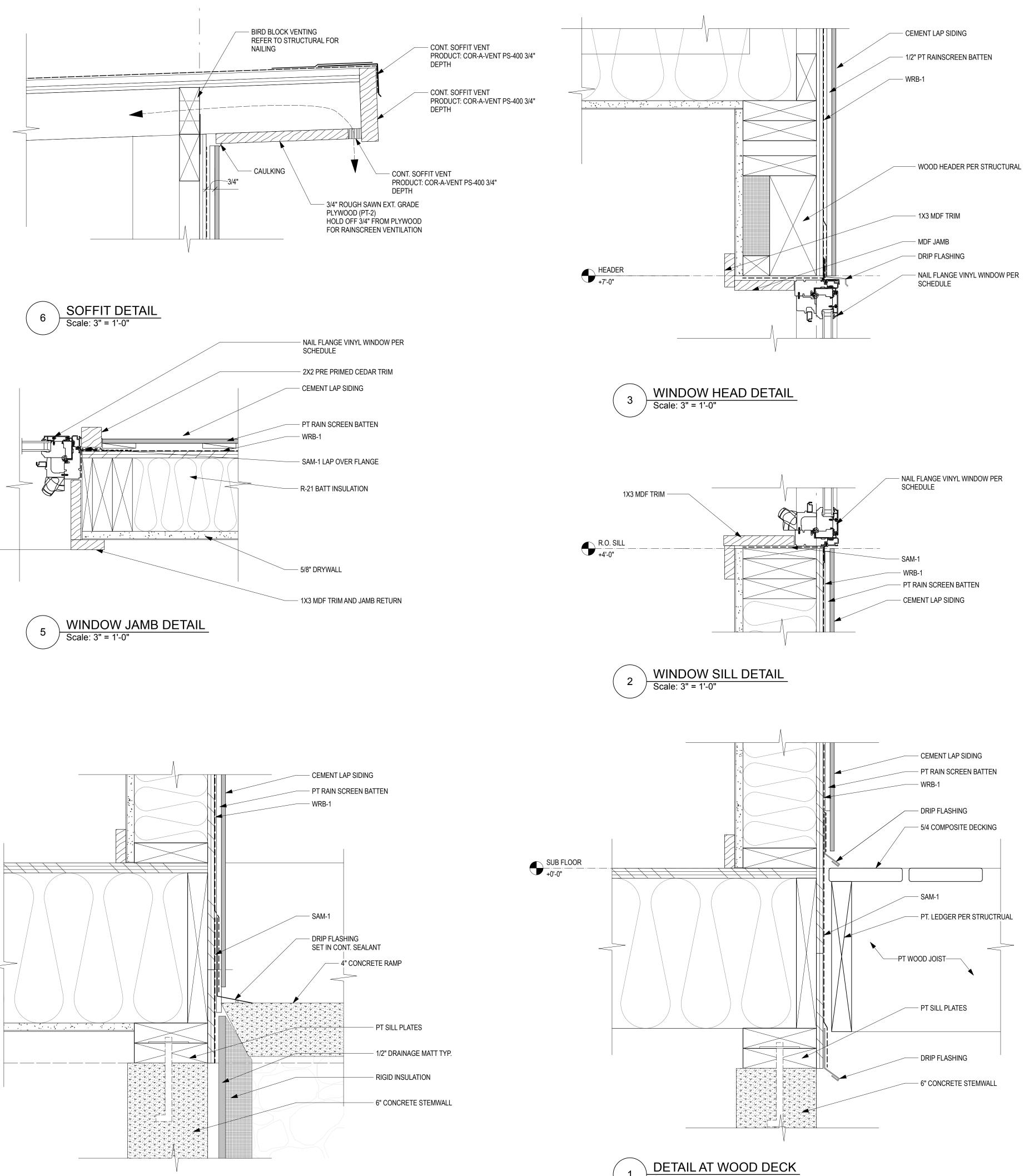
1 DETAIL AT WOOD DECK Scale: 3" = 1'-0"
