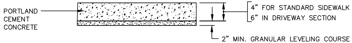
SIDEWALK SURFACING DETAIL
