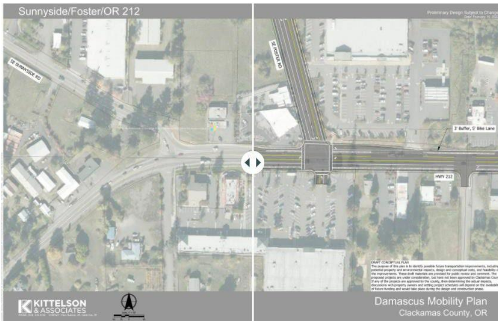
Restrict movements at OR 212/SE Sunnyside Road-Anderson Road and provide additional lanes at intersection of OR 212/SE Foster Road (Regional Project)
