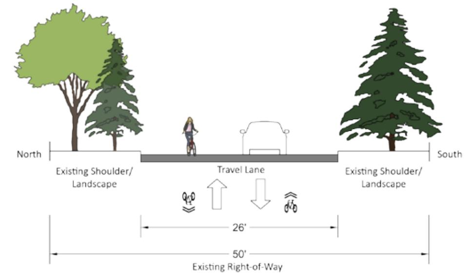
Figure 4.23 Proposed cross-section for Boyer Drive, between 82nd Avenue and the I-205 Multi-Use Path
