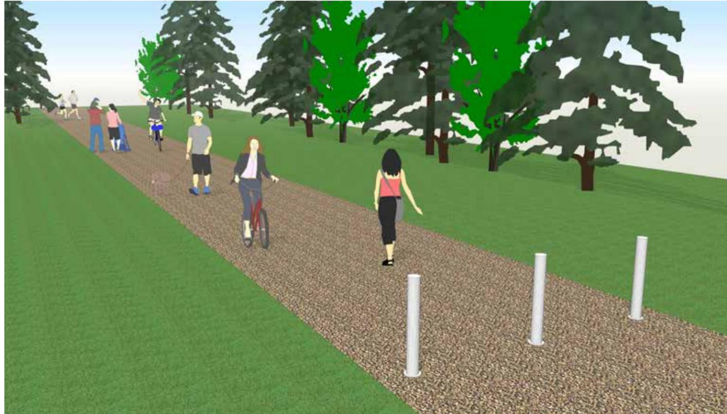
**Figure 4.11** Conceptual rendering of Monroe Gap. Bollards prevent automobiles from driving through while preserving emergency vehicle access. The 12-foot path is bordered by natural landscaping on both sides.
