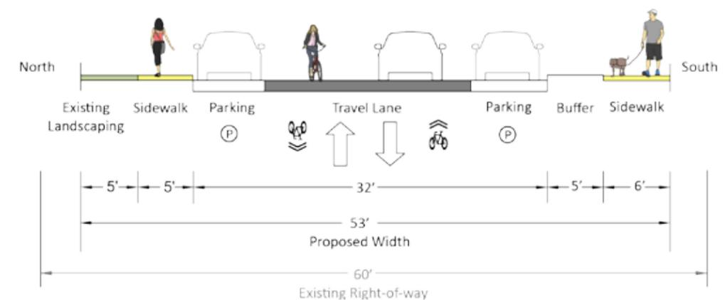
Figure 4.11 Proposed cross-section for Monroe Street, between 77th Avenue to Fuller Road (east of the Monroe Gap)
