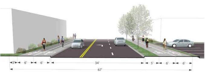
**Figure 4.19** Cross-section for Boyer Drive Extension, between Fuller Road to 82nd Avenue
