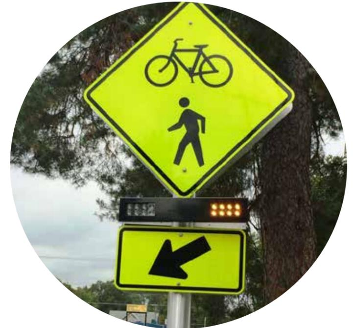
Example of a rapid-flashing beacon. Photo: City of Lincoln, NE Traffic Engineering
