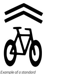
"Sharrow" pavement marking, used to indicate a street environment shared by bicyclists and automobiles. Image: CH2M (2016).
