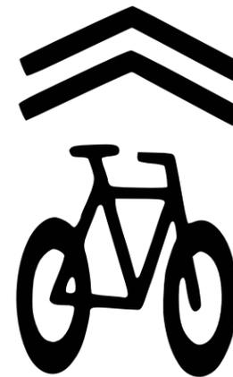
Example of a standard “sharrow” pavement marking, used to indicate a street environment shared by bicyclists and automobiles. Image: CH2M (2016).
