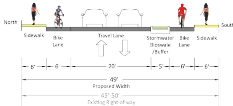
Figure 4.17 Proposed cross-section for Thompson Road, between 74th Avenue and Fuller Road
