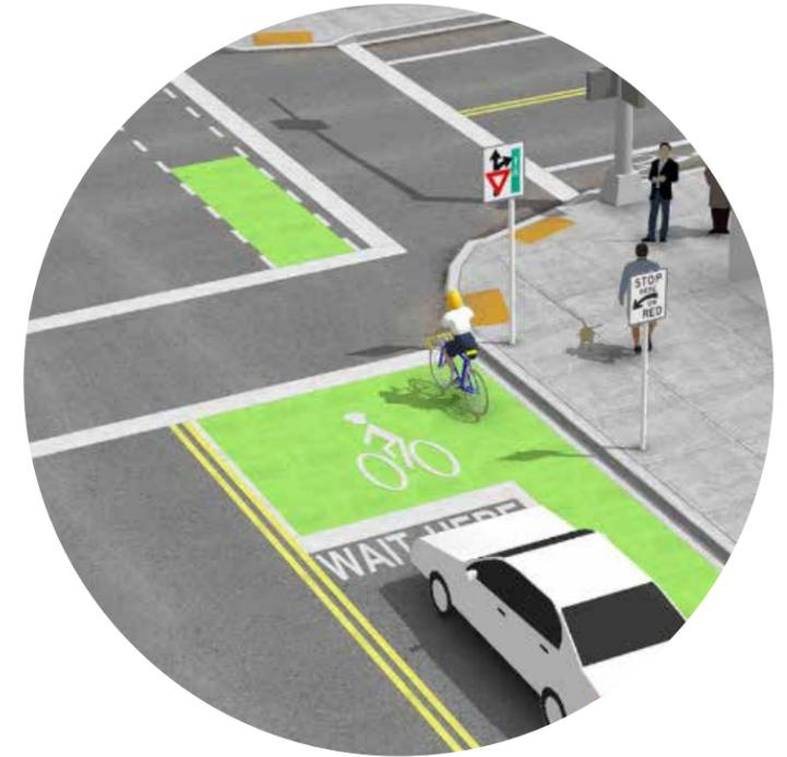
Conceptual rendering showing a bicycle box at a signalized intersection with a bicycle lane approach. Credit: NACTO (2015)
