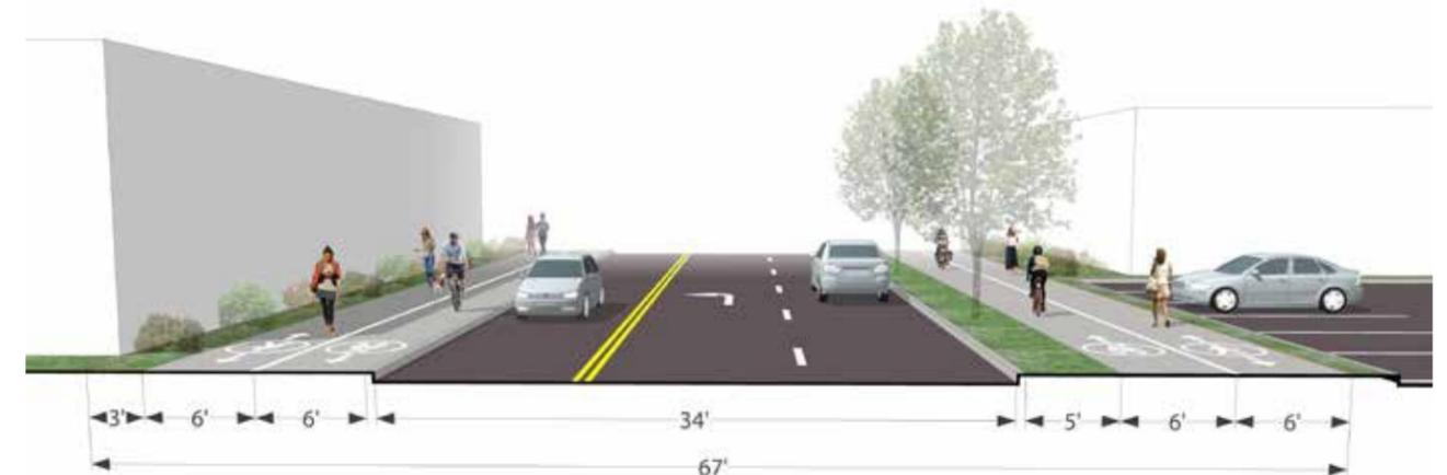
Figure 4.19 Cross-section for Boyer Drive Extension, between Fuller Road to 82nd Avenue
