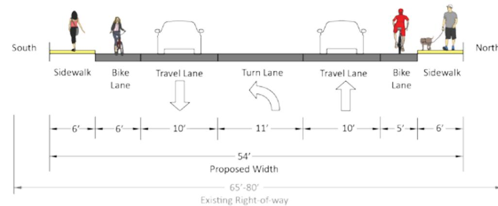
Figure 4.21 Proposed cross-section for Boyer Drive, between 82nd Avenue and 85th Avenue
