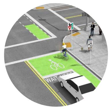
Conceptual rendering showing a bicycle box at a signalized intersection with a bicycle lane approach. Credit: NACTO (2015)
