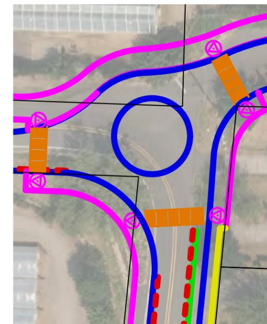
**Figure 4.5** Enlarged recommended design for intersection
