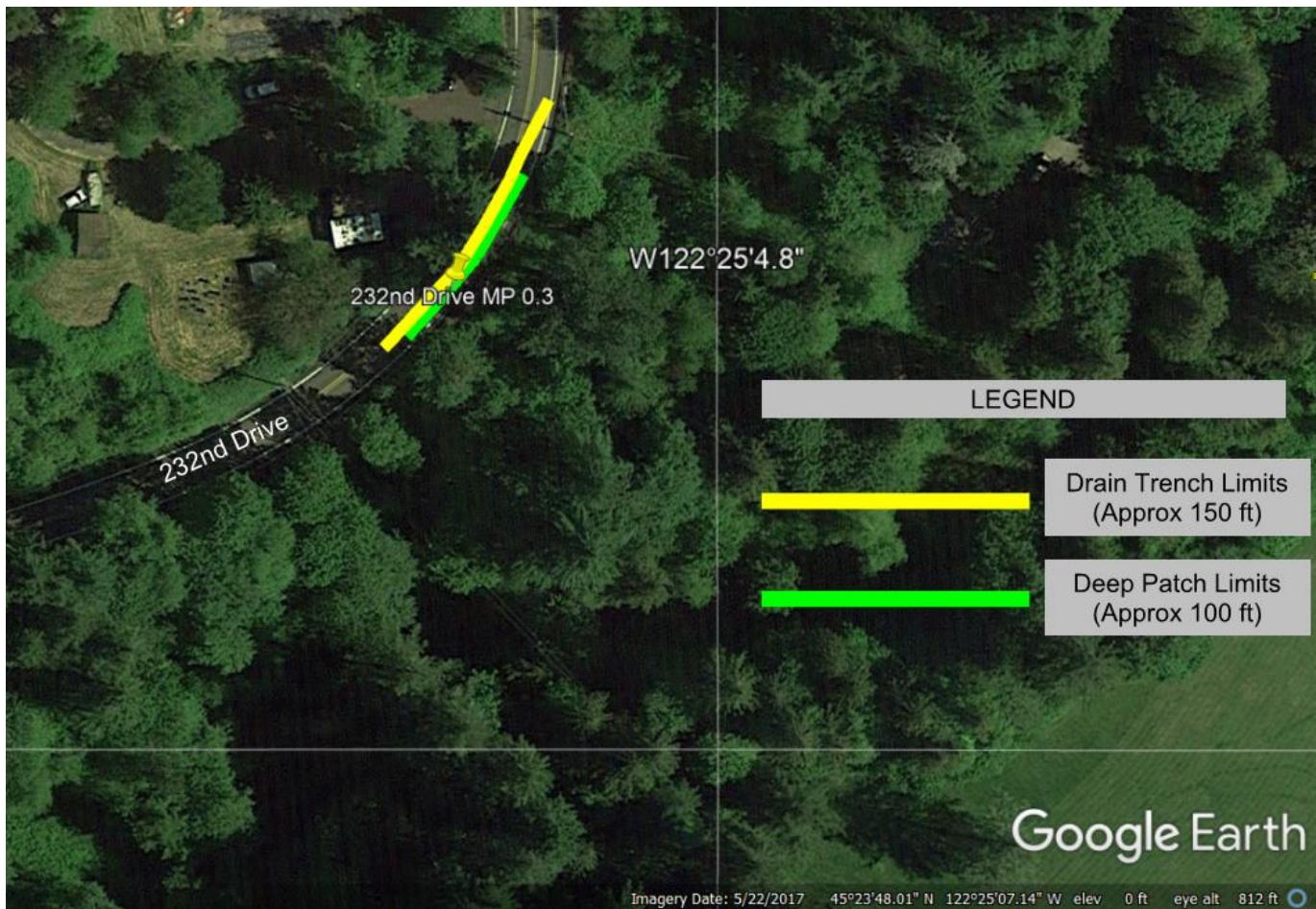
Figure 1 – Approximate limits of improvement for the Project.
