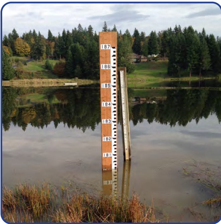
Image 7: New staff gage installed for client in Clackamas County to quickly reference lake water levels.
