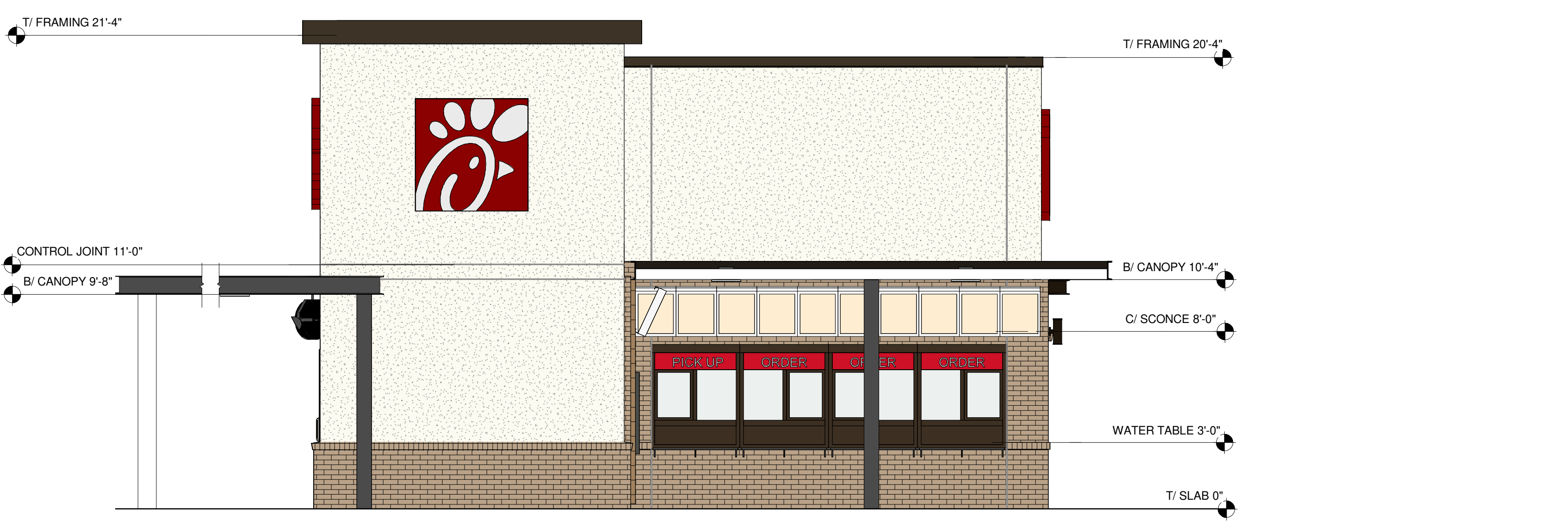
B2 NORTH EXTERIOR ELEVATION 1/4" = 1'-0"
