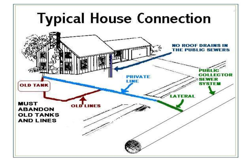
The **building sewer** is that section of pipe beginning 3 feet outside the foundation of the house (shown in blue above) and running to the point of connection with the Public Collector Sewer called the service lateral (shown in green above).
