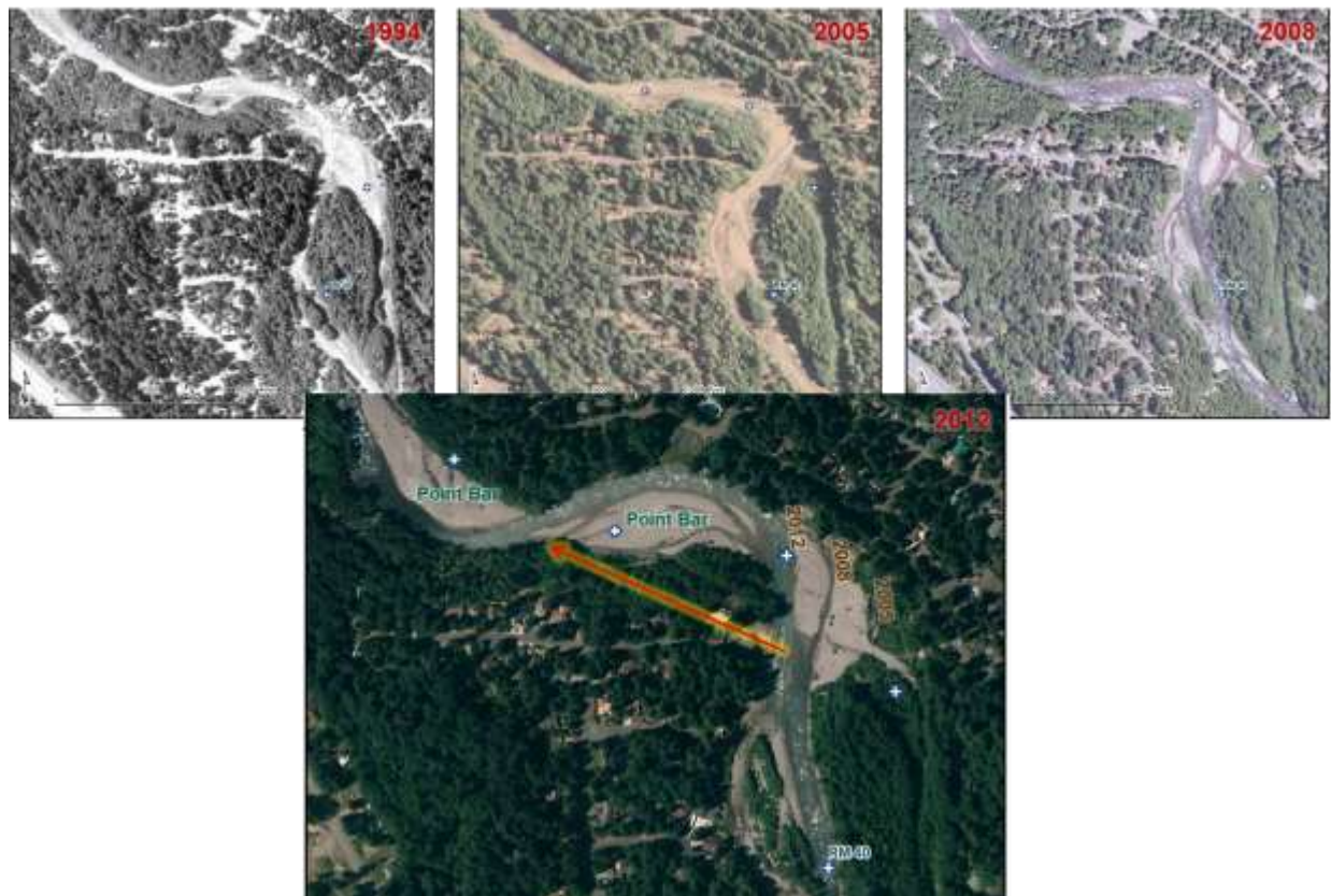
Figure 23. Timberline Rim Channel Migration. This group of air photos shows the lateral and downstream migration of the large bend adjacent to the Timberline Rim community. Note the remnant channel traces showing the distance of migration from 2005 to 2008 to 2012. Note also the size of the bend relative to property plats. Data sources: University of Oregon Libraries, USDA NAIP.
