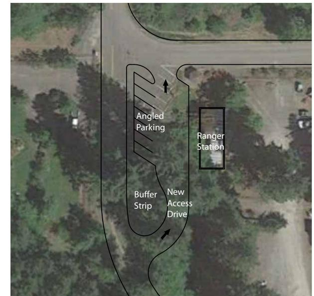
*Figure 5-1. New Circulation at Ranger Station*
